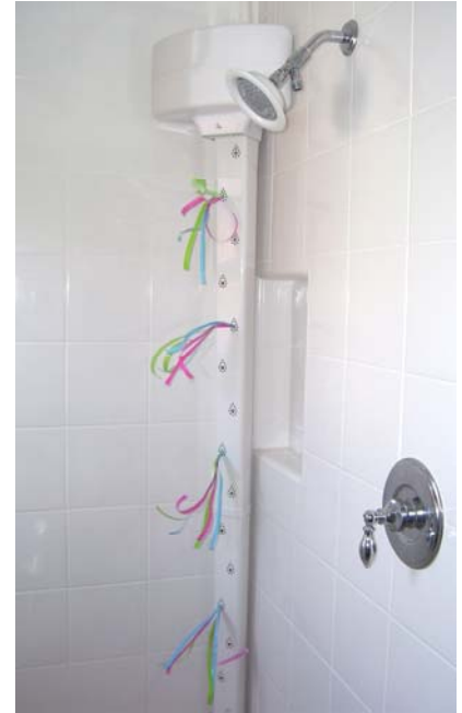
Streamers Added to Show Air Flow
